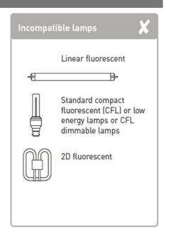
This product requires a minimum load of 60W. Therefore it may not be suitable for use with low power lighting such as LED. If you wish to use less than the minimum load specified, please see below:
